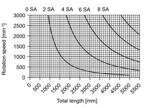
For mechanical linear drives with roller guide, the static load rating " $C_{stat}$ " (page TL 11) applies for static loads. Special design: Spindle support with damping ring (extension of total length: 10 mm for every 2 SA) Design with double nut ("MM") is only available with long carriage plate 270 mm and pitch "5", "10" oder "20".
