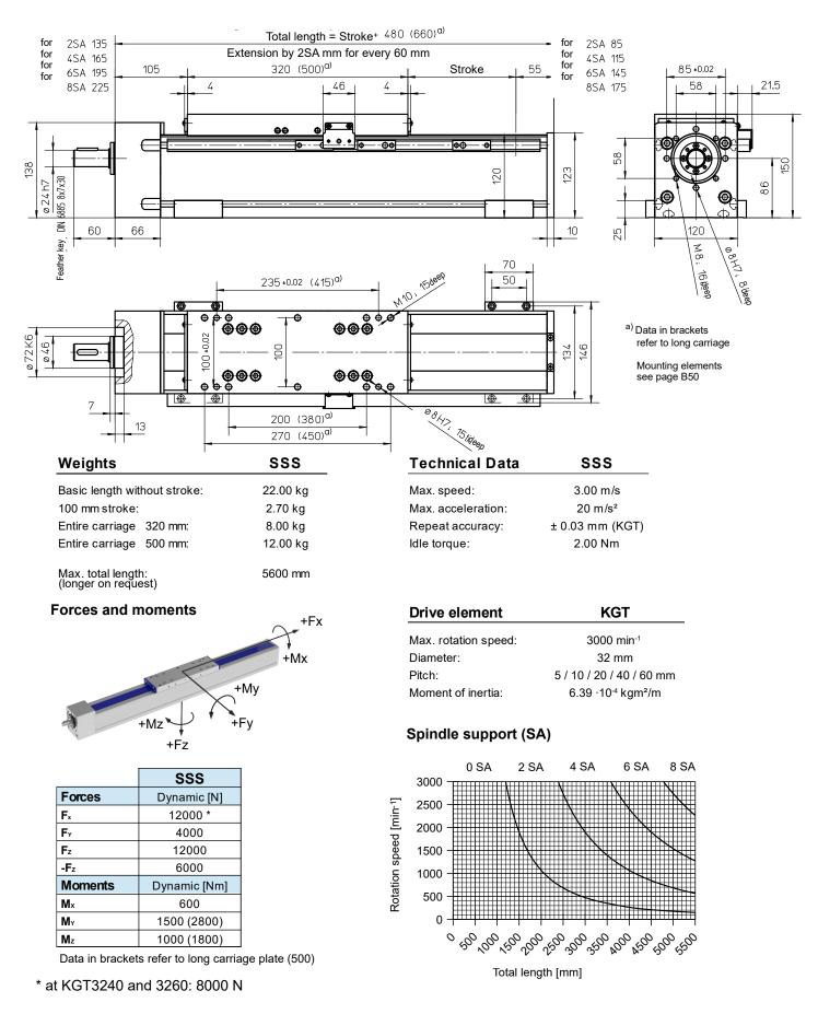
Special design: Spindle support with damping ring (extension of total length: 10 mm for every 2 SA) Version with double nut ("MM") only available with long carriage (500 mm) and pitch "5", "10" or "20".
