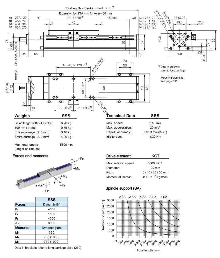
Special design: Spindle support with damping ring (extension of total length: 10 mm for every 2 SA) Version with double nut not possible.
