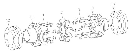
Illustration 17: ROTEX® GS clamping ring hub
