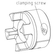
Illustration 20: Assembly of clamping hub
