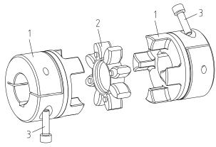
Illustration 14: ROTEX® GS clamping hub
