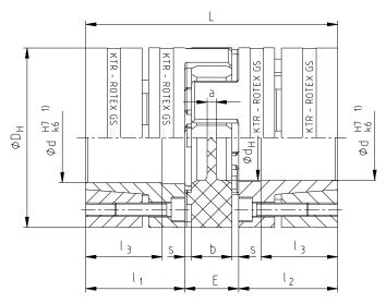
Illustration 9: ROTEX® GS, clamping ring hubs
