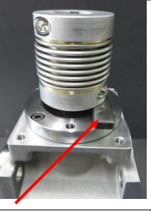
Fit coupling, prepare, as described above. If prescribed, set mounting dimension of the coupling, in accordance with dimension sheet. Tighten clamp screw.
